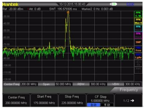
6. Press [AMPT]  $\rightarrow$  Attenuation  $\rightarrow$  10dB to turn up the RF attenuation to 10 dB.
