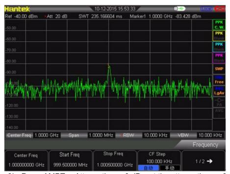
3) Press AMPT  $\rightarrow$ Attenuation $\rightarrow$  0 dB, set the attenuation as 0 dB.
