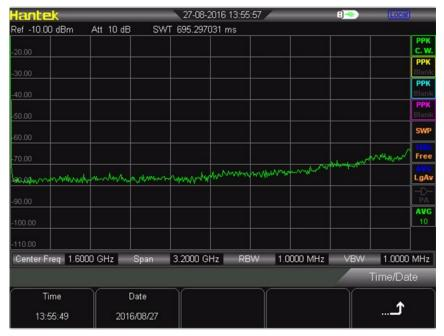
The system time is displayed in "hh:mm:ss YYYY-MM-DD" format in the DSA800 user interface. The output file can include the time information when printing or storing interface image according to your setting.
